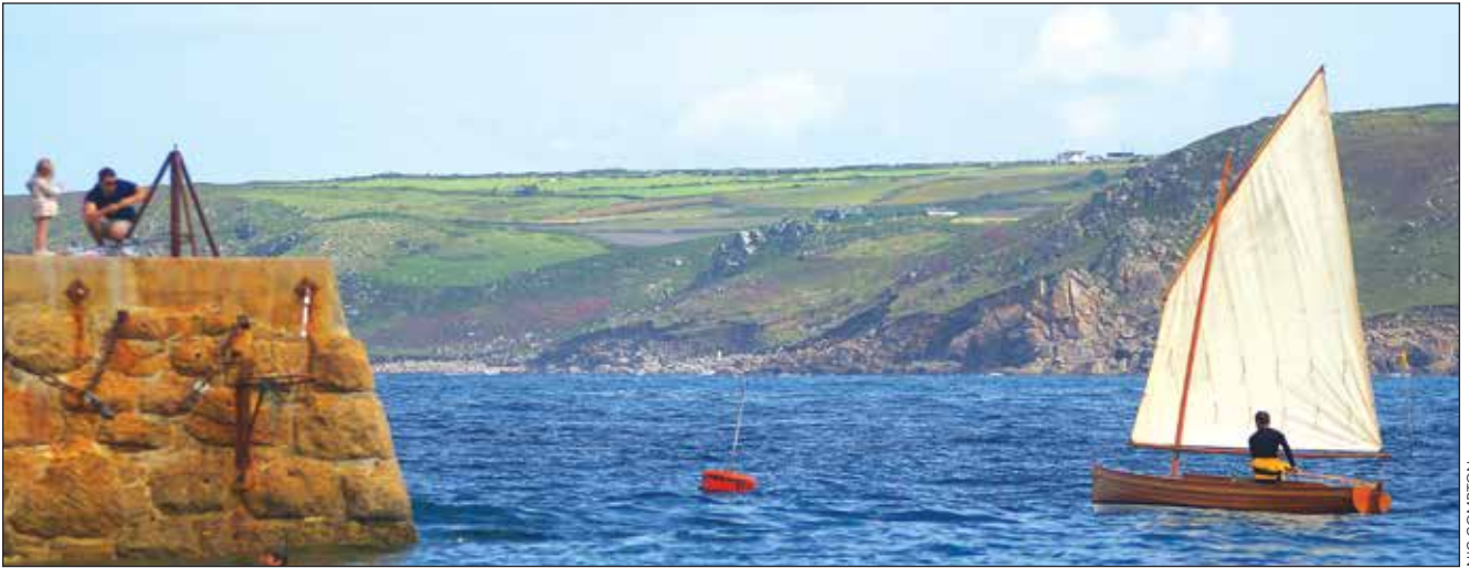
Will Stirling’s 15’ Sailing Dinghy is designed for coastal expeditions. Its long foredeck and wide side decks help keep the spray out of the cockpit. The balance lug sail works well on all points of sail, except close-hauled.
